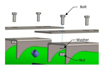
2. Mount the compressor on top of the pressure vessel using a gantry. Compressors range in weight from 95 lbs to 880 lbs. Use extreme caution and avoid injury.
