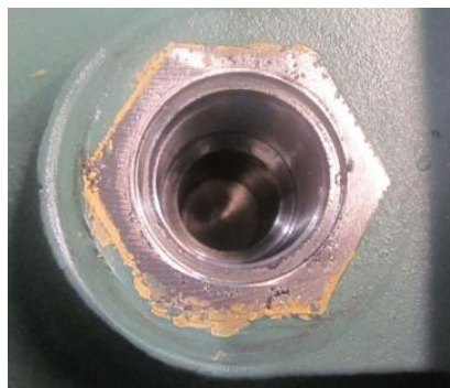
Stator Pin Recess shown with O-ring
