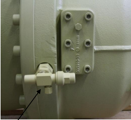
Shut-off valve for Liquid Injection
