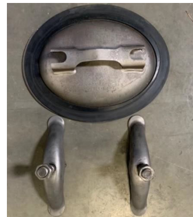
Figure 1 Manway Cover Showing Gasket Bitzer P/N P000014995
