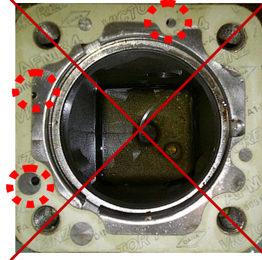
Example of Incorrect Gasket Installation
