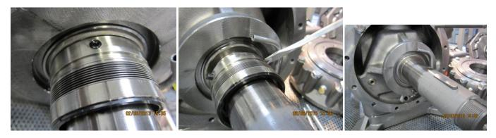
4. Oil the new shaft seal, the o-ring area on the housing cover, the sealing cover and the gaskets. Torque the shaft seal set screws to 4 Nm (hand tight); the housing cover bolts to 125 Nm and the sealing cover bolts to 40 Nm.
